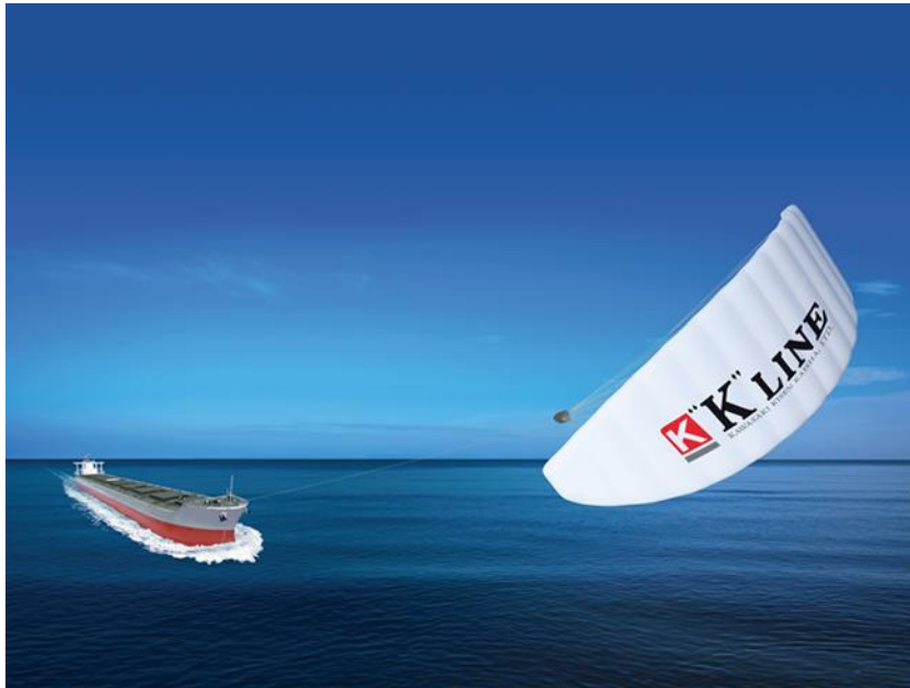
Image of Seawing Installation
